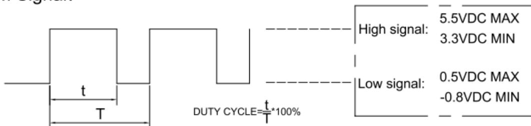
1.The control signal frequency of the fan shall be able 18KHz~25KHz.
